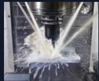
Mist / Flood Cooling
